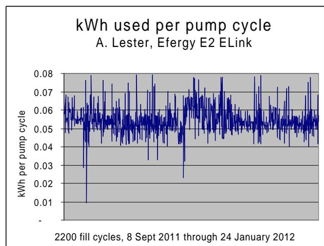
\* “Use of a smart header tank which is refilled only when it's nearly empty reduces use of the pump such that the average cost of electricity for the pump is less than 1 penny per person per day”
