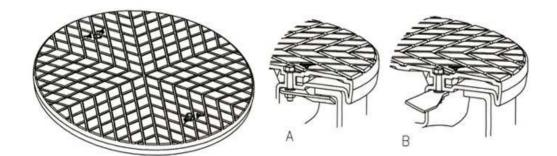
A Safety latch closed B Safety latch opened
