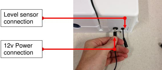
MAKE SURE THE FLOAT SWITCH IS CONNECTED <u>BEFORE</u> THE POWER IS SWITCHED ON Connect the unit's 12 volt DC adapter to a 220V AC mains socket. Power should be maintained to the unit at all times.
