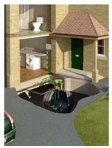
The Rain Backup in a Box® is fitted inside the building where the occupiers can see and hear it. When rainwater has run out in the underground tank, a float switch that is in the underground tank will drop and open the solenoid valve. Mains water will flow to the tank and put a small amount of water into the tank to ensure that the pump keeps running.
